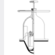
Non-rising handwheel with indicator DN200 - DN300 8" - 12"
